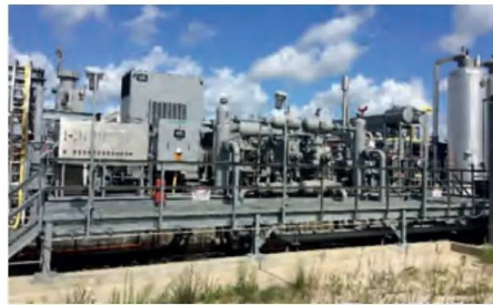
FIGURE 7 Reciprocating compressor package at an underground hydrogen storage facility in Texas, USA 8
